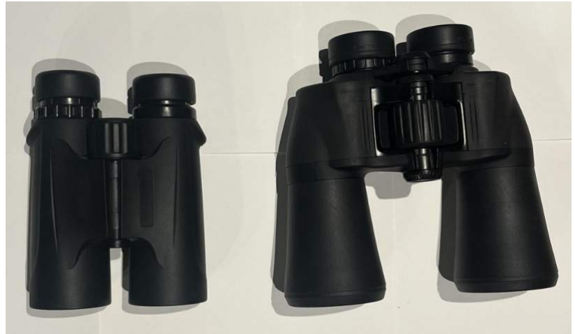
THE TWO MOST POPULAR TYPES OF BINOCULAR DESIGNS ARE SHOWN HERE: ROOF-PRISM BINOCULARS (LEFT) AND PORRO-PRISM BINOCULARS (RIGHT).
