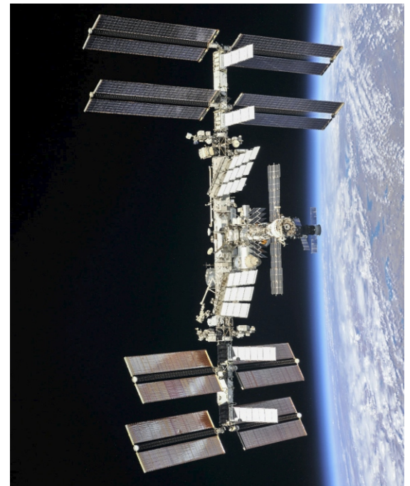
A complete view of the ISS as of October 4, 2018, taken from the Soyuz capsule of the departing crew of Expedition 56 from their Soyuz capsule. This structure was built by materials and 5 Russian Proton and Soyuz rockets, and assembled into orbit by 37 United States Space Shuttle missions and maintained by 230 spacewalks, with more to come! Credit: NASA/Roscosmos More info: bit.ly/issbasics
