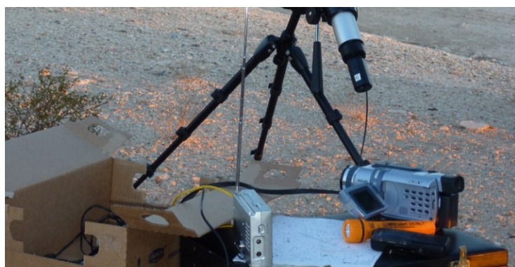
Typical 80mm telescope set up with older style camcorder and radio (no longer used)
