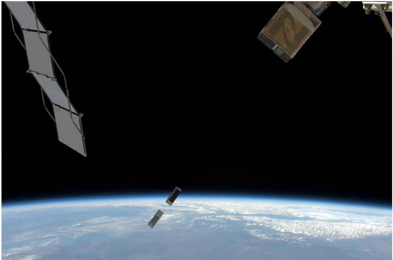
Astronaut Tim Peake on board the International Space Station captured this image of a CubeSat deployment on May 16, 2016. The bottom-most CubeSat is the NASA-funded MinXSS CubeSat, which observes soft X-rays from the sun—such X-rays can disturb the ionosphere and thereby hamper radio and GPS signals. (The second CubeSat is CADRE—short for CubeSat investigating Atmospheric Density Response to Extreme driving - built by the University of Michigan and funded by the National Science Foundation.) Credit: ESA/NASA
