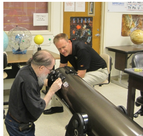
Don assisting Marcus Hermann with collimating his 10" Orion Intelli-scope at the PVCC Telescope Workshop. Photo by Terri.
