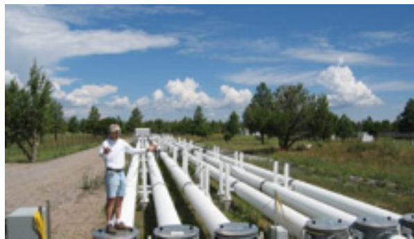
Nat shows us the “delay line” pipes that allow them to fine tune the interference images obtained. The pipes contain a vacuum to minimize light scattering.
