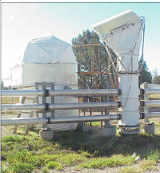
Interferometer Tour. This is one of the light collecting units at the Interferometer up on Anderson Mesa. The unit on the right sheds its lid and collecting the photons, which then sends them down the white tube and into one of the three silver horizontal tubes via mirrors.
