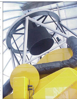
This is the smaller scope within the dome along side the main dome's location at the Naval Observatory. it is cooled with liquid nitrogen and has a massive unit on the bottom where the CCD camera is connected. Ron Stone showed us this wonderful scope. The dome was kept mostly closed due to threatening clouds.
